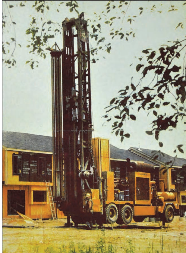
Figure 7.4: A Down-the-Hole (DTH) Rig
