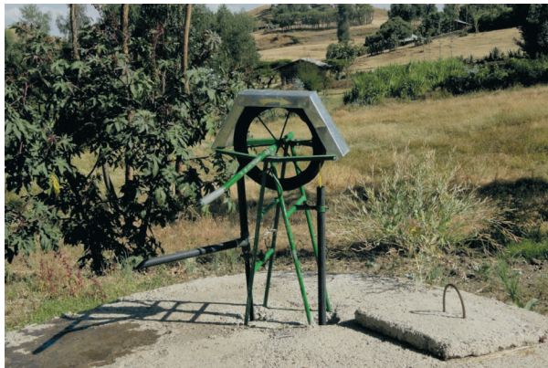
FIGURE 4 ROPE PUMP (PROTECTED HAND-DUG WELL)
