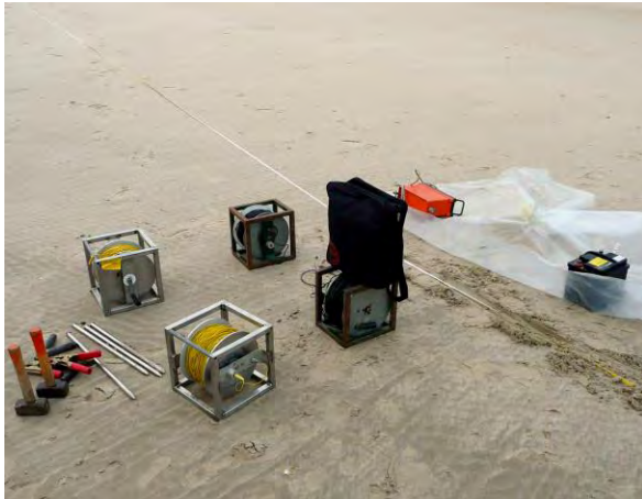
Figure 14: Set up of a VES measurement at the beach. Four reels of wire are used to connect the measurement unit (the orange device) to the current and potential electrodes.
