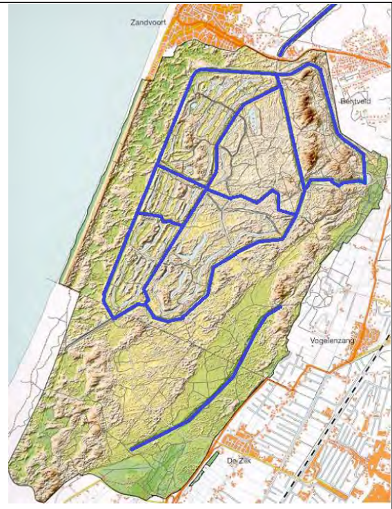
Figure 52: Example of a dune water system with infiltration basins, at the Amsterdam Waterworks, The Netherlands.
