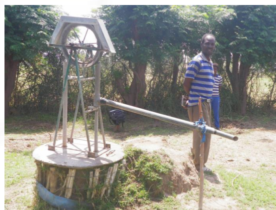
Figure 6. Mr. Girma Bulfato next to his hand dug well equipped with rope and washer pump.
