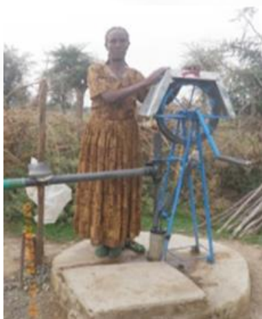
Figure 3. Ms. Kebebush Ergicho and her manually drilled well with rope and washer pump.
