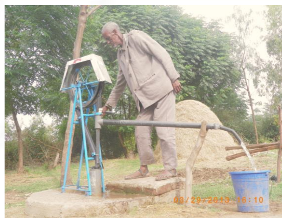
Figure 2. Mr. Bejiga Chali pumps water from the manually drilled well with a rope and washer pump.
