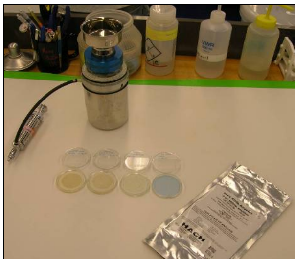
Figure 5.2 – Membrane Filtration apparatus (Mattelet 2006)
