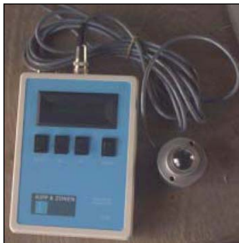
Figure 5.7 - Solar radiation measurement apparatus (Oates 2001)
