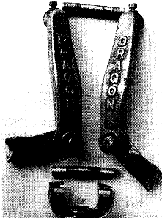
Wear on the handle fork resulted in breakage of the iron casting.
