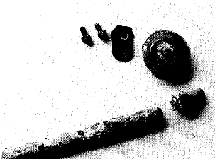
Corroded and worn foot valve components which resulted in breakage of the plunger rod.
