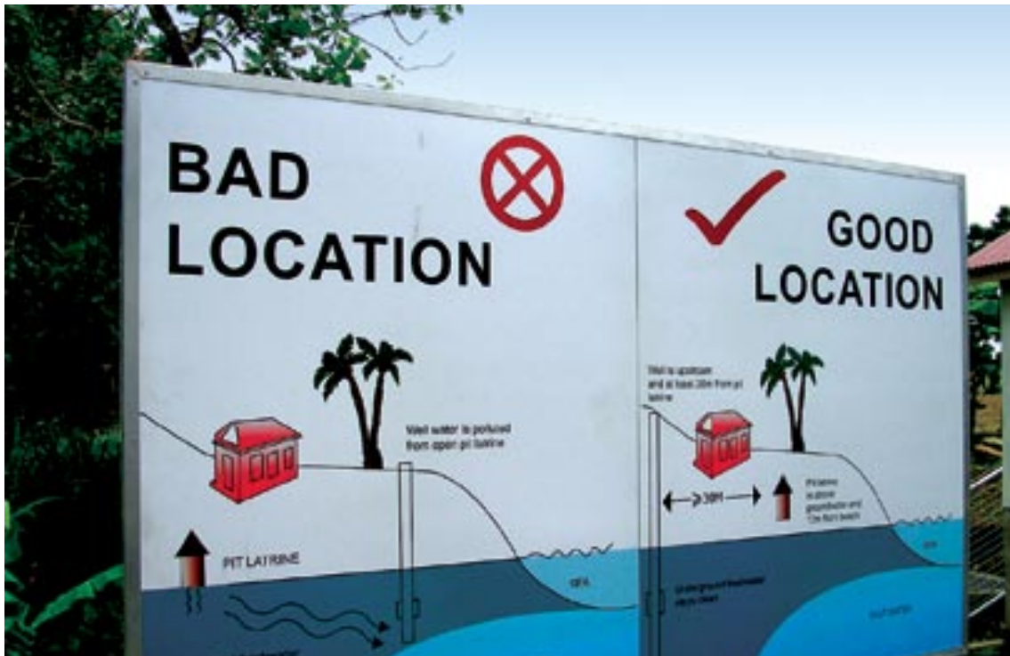
Signage on good and bad location of a pit latrine
