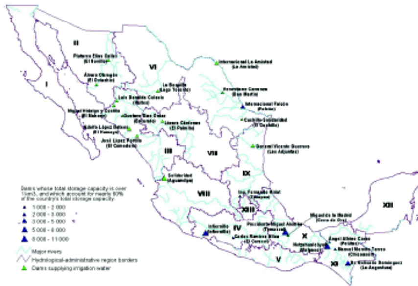
Dams accounting for nearly 60% of the country's total storage capacity
