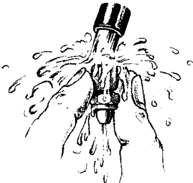
Fig. 9.18. Clean the nozzle tip with water (© WHO).
