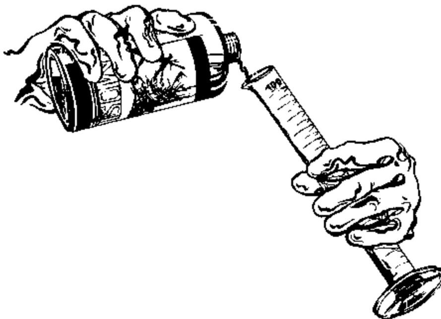
Fig. 2.24. The insecticide emulsion is measured with a measuring cylinder.
