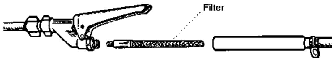
Fig. 9.17. Removing the spray filter for cleaning (© WHO).
