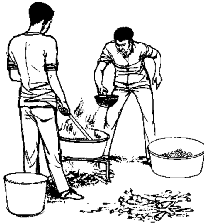
Fig. 1.101. Unexpanded polystyrene beads can be expanded near the site of application in boiling water in a cooking pot.
