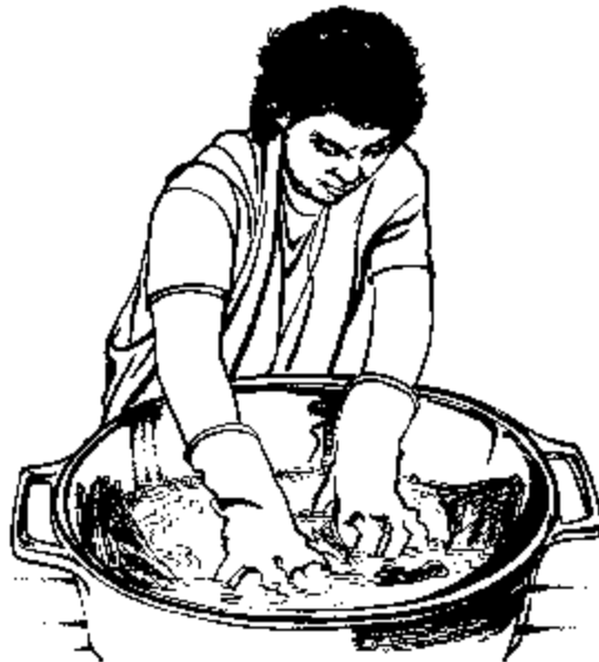
Fig. 10.13 Wear long rubber gloves and use a wide, shallow bowl when impregnating fabrics.
