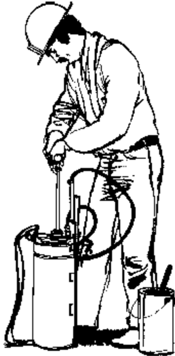
Fig. 9.12. Pressurizing the spray tank.
