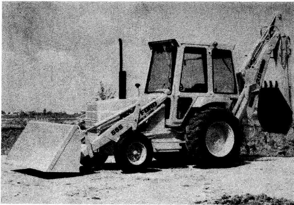
Fig. 6. Wheel excavator (backhoe)-loader, mounted on a farm tractor.
