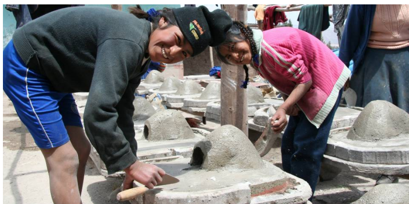
Making pourflush bowls as part of a sanitation marketing initiative supported by WSP, USAID, and others in Peru. (photo: WSP)
