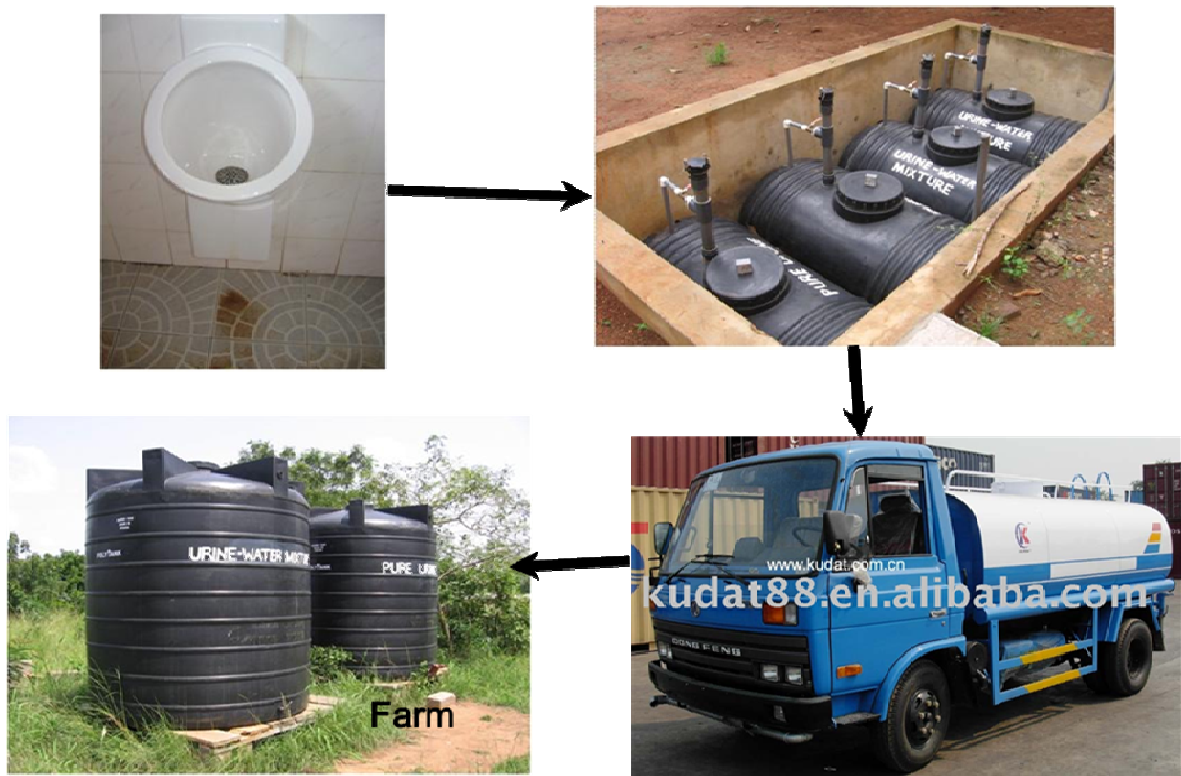
Figure 6-4 Infrastructure required for urine harvesting and application
