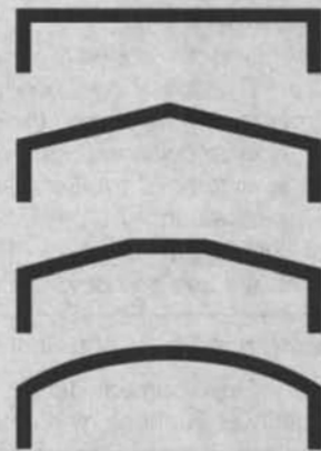
Roof shapes - sectional view
