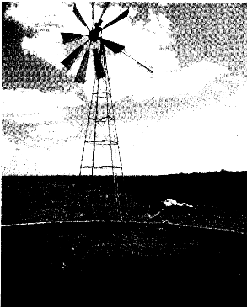
Monitoring in actual use. Storage tank as 'interface' between windmill and user (Cattle ranch of Mr. Alberto Soares, owner of Mapel wind pump factory, Salvador, Brazil).
