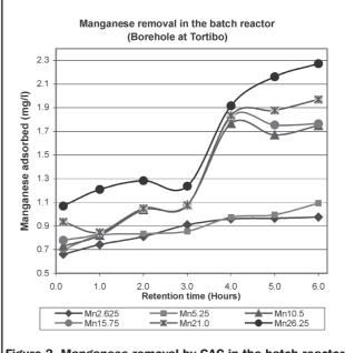
Figure 2. Manganese removal by GAC in the batch reactor for water sample from Tortibo.
