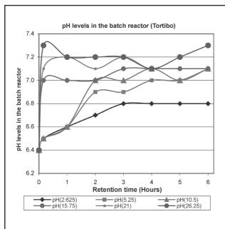
Figure 4. pH levels in the batch reactors for water sample from Tortibo.
