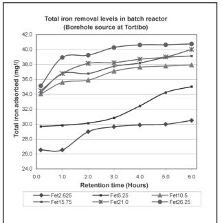
Figure 3. Total iron removal by GAC in the batch reactor for sample from Tortibo.
