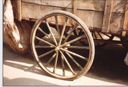
Locally made in Delhi. Strengthened wheel using iron tubing as spokes. Note the radial arrangement of spokes, and flat tyre.
