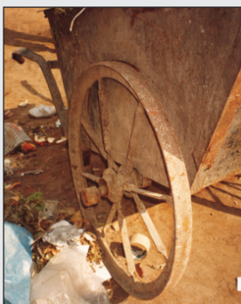
An iron wheel on a handcart in Delhi. The combination of solid wheel and poor bearings would make this a difficult cart to use.
