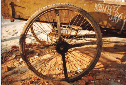
Reinforced bicycle wheel on a cycle cart in Delhi. Note the smaller tangentially arranged spokes.
