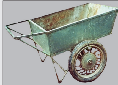
Simple handcart with motorcycle wheels, Lusaka
