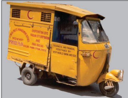
Motor rickshaw adapted for hospital waste collection in Dhaka
