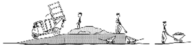
Figure 6.3: Sorting on a platform. Waste is delivered onto the platform. Workers stand upright and sort out organic waste and fill it into wheelbarrows below. Advantage: no further need for shoveling and no direct contact with the waste
