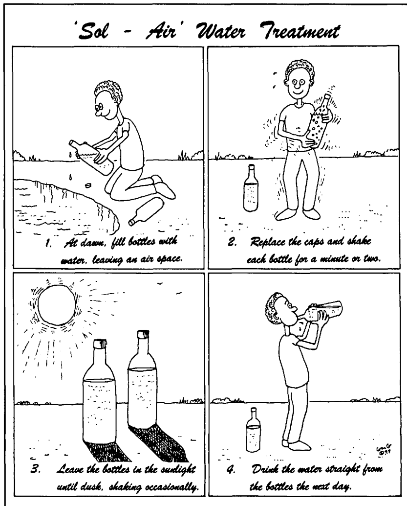
Figure 2. The four stages of solar photo-oxidative disinfection.
