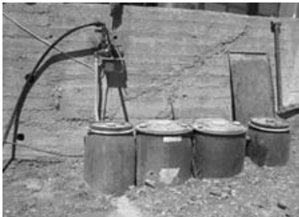
Figure 9: Four-Barrel Upflow Gravel Filter.
