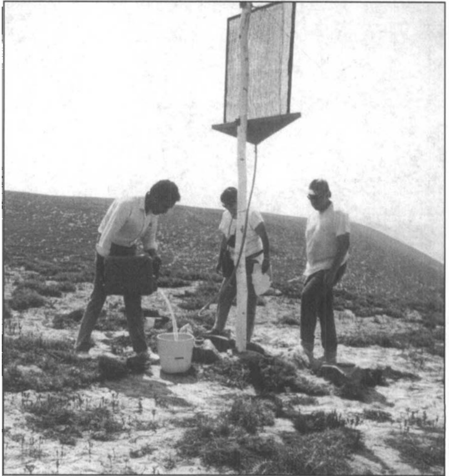
Fogwater being collected in a mining area 250km south of Lima. Pollution has affected the natural colour of the lomas, and the fogwater shows a high concentration of iron. It can be purified by filtration.
