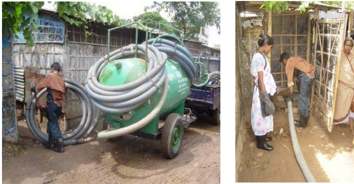
Figures 10 and 11 : The Vacutug being used to desludge a cesspool
