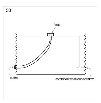
**33.** If settling water with a high concentration of suspended sediment, a layer of sludge will accumulate in the bottom of the tank. The cleanwater outlet is then best connected to a length of green flexible hose, hanging from a float. This will reduce flow, but it has the benefit of keeping discharge flow more uniform. The other low-level hole is then used only for desludging. Alternatively, the outlet hole sheet can be fitted
