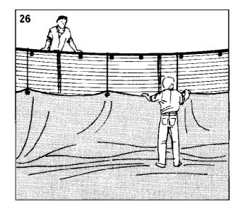
27. Continue to lift the liner, working from a platform of about half the height of the tank, taking care to protect the liner from the pressure of the platform. Continue until the liner has passed over the top and a short distance down the outside.
