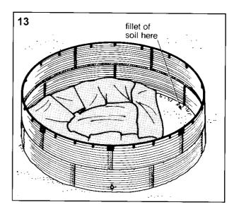
14. At this stage ensure that the vertical seams in the liner do not coincide with any of the holes in the tank sheets. If they do, rotate the liner base slightly. Lift the liner over the rim without disturbing the protective PVC capping. You now need many helpers on the outside, to hold the liner and prevent it slipping back inside, while adjustments are made to minimise wrinkles and to end up with an equal margin hanging down all around outside.
