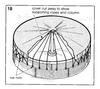
**19.** When the tank is in use, an inspection flap which is provided in the PVC roof near the tank edge and can be used for dosing chemicals, insertion of delivery pipe or inspection of the tank. Finally, either tie ten guy ropes to eye bolts spaces around tank and peg down, or bank earth against outside of tank to 1/3 of tank height.
