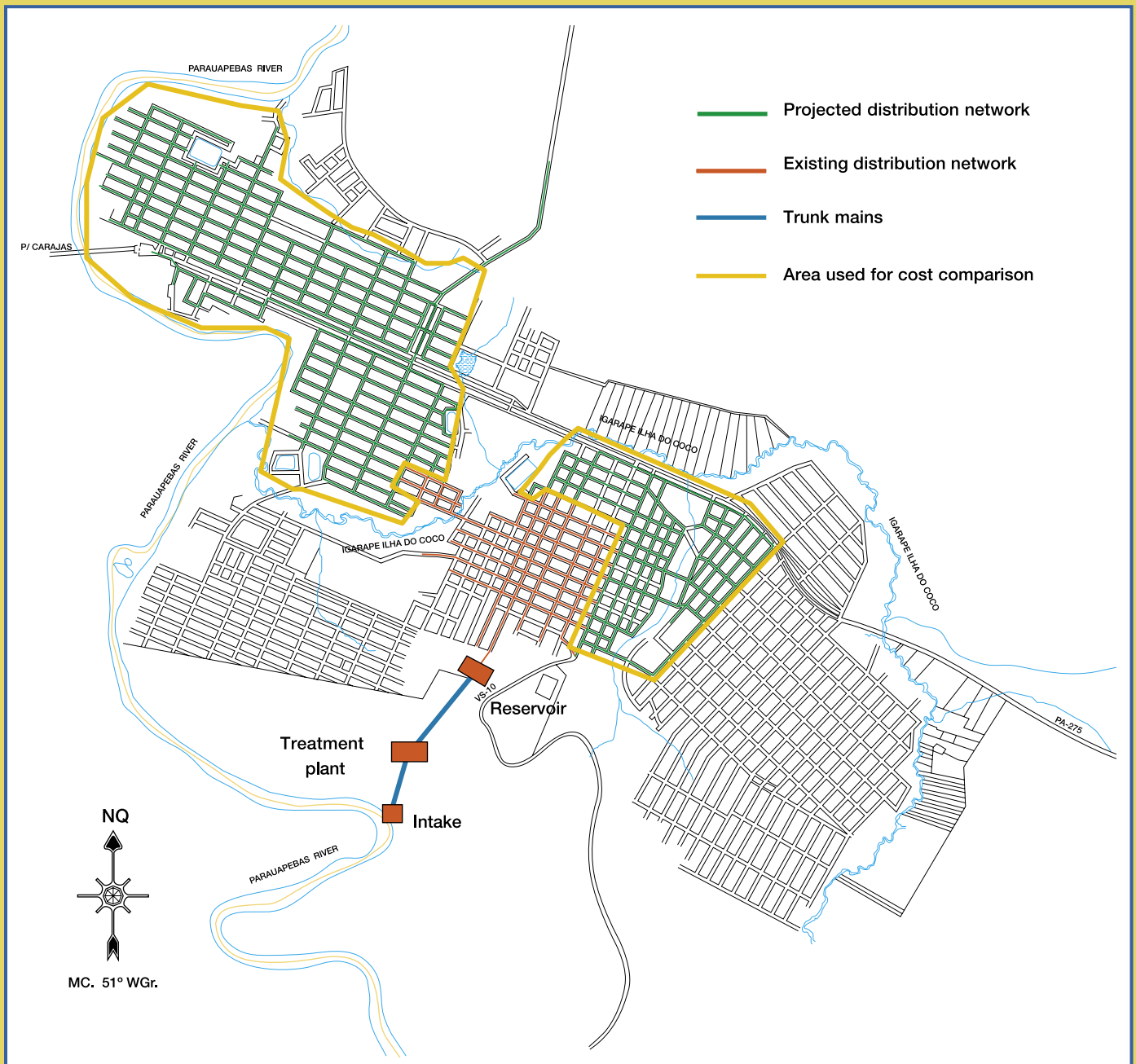
Figure IV.1: Original conventional water system design for Parauapebas
