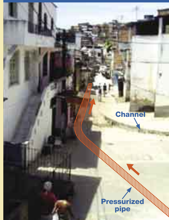
Illustration of the area requiring pressurized sewers
