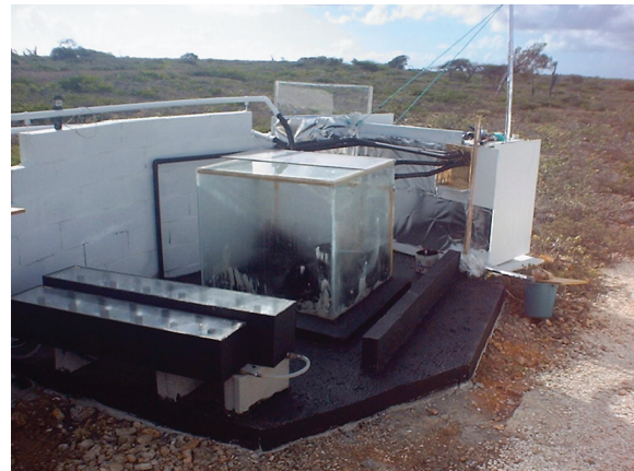
Fig. 4. Real world look of the working prototype producing 40 l freshwater per day; the industrial design will include all components in one compact cubicle.
