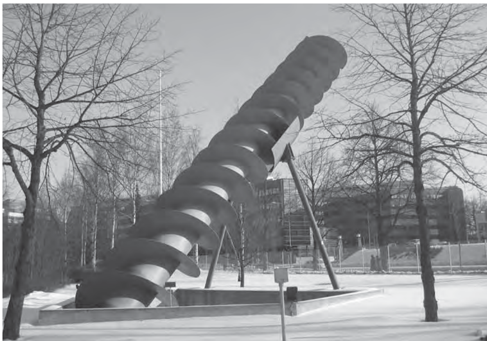
Plate 66. Example of technology used for 2,000 years: an abandoned large-size archimedes screw pump in Tampere, Finland used now as a statue. Similar pumps are still commonly used worldwide for pumping raw sewage and sludge (Photo:T. Katko, 2005)
