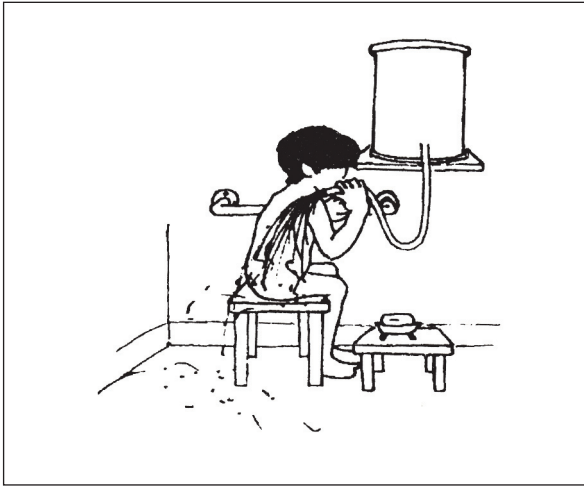
Figure 6.70. Bathing with a flexible hose connected to a water container.
