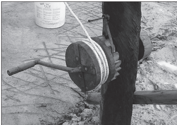
Figure 6.9. Detail of ratchet and pawl winding mechanism.
