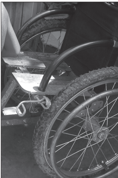
Figure 9.75. Wheelchair seat with central plank removed.
