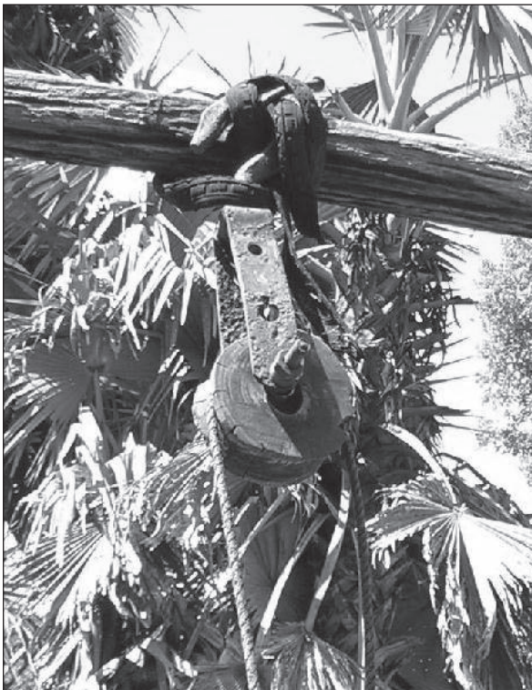
Figure 6.8. Detail of pulley lifting mechanism. (Case-study 9.12, page 191)
