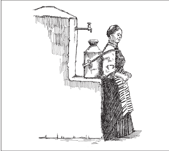
Figure 6.13. Tapstand in Tibet with higher tap and shelf that does not require the user to bend. (Case-study 9.32, page 252)
