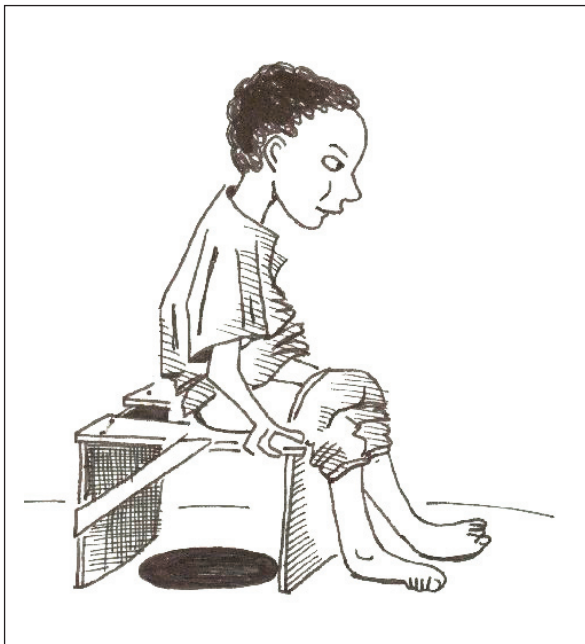
Figure 7.35. Wooden toilet stool for use over the family pit latrine. Gap between planks: 10cm – suitable for a child. Front plank acts as splash-guard.
