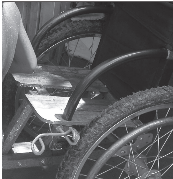
Figure 7.40. Wheelchair with a centre plank removed to leave a gap in the seat for toileting.* (Case-study 9.15, page 201)
