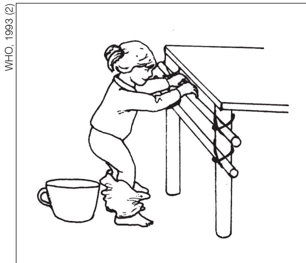
Figure 7.10. 'Ladder' of rails to help a child pull herself up and lower herself down.
