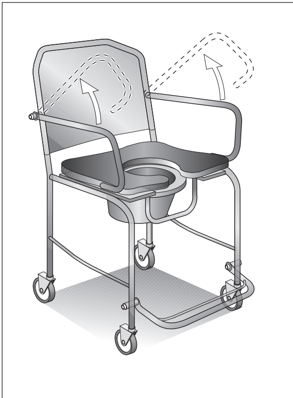
Figure 7.21. Chair with side-rails that can be raised. The rails are attached to the chair back with a bolt, on which they swivel vertically.
