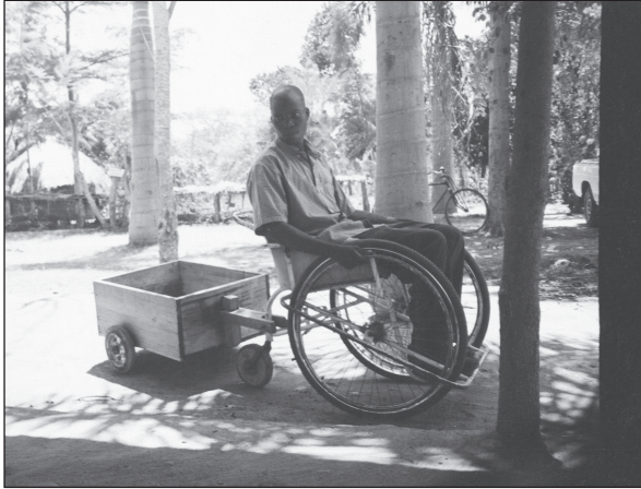
Figure 6.29. Two-wheeled wooden wheelchair trailer.
