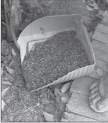
Figure 9.90. Ash scoop made from an old jerry-can.
