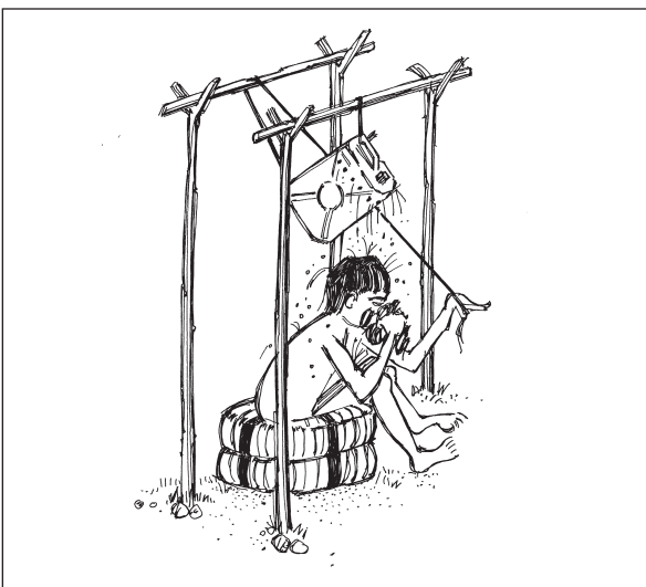
Figure 6.65. Adapted jerry-can with holes pierced around top. (Case-study 9.27, page 237)
