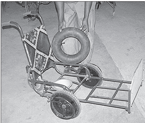
Figure 7.49. The low trolley has a pot that fits into the frame under an inner tube, which functions both as a cushion and as a toilet seat. For general use, the inner tube is covered with a mat.
