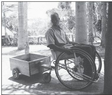
Figure 9.150. Two-wheeled wooden trailer.
