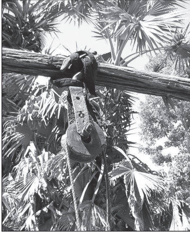
Figure 9.52. Locally made wood and metal pulley.
