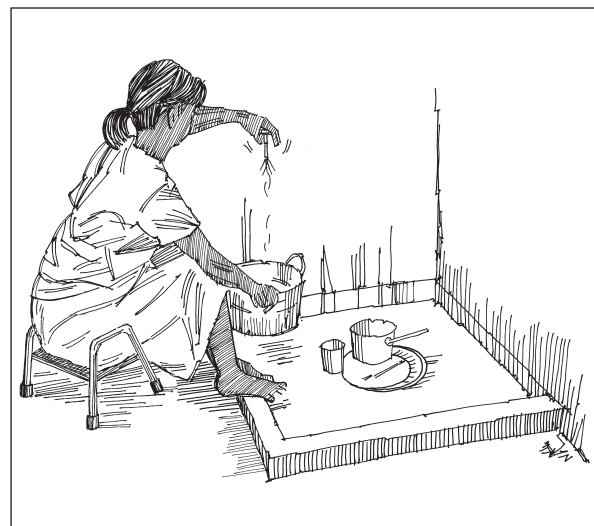
Figure 6.86. A floor level dish-washing facility in the corner of the kitchen. (Case-study 9.4, page 169)
