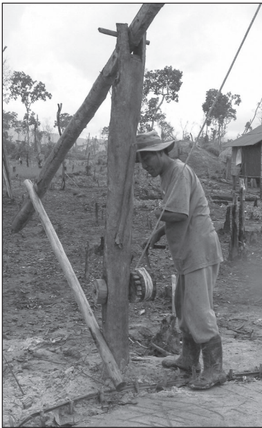
Figure 9.48. Mr Ath turns handle of winding mechanism to lower and lift bucket.
