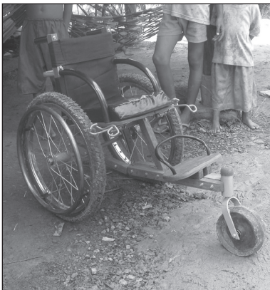
Figure 9.74. Mekong wheelchair with foot-rest, also used as a transfer-seat.
