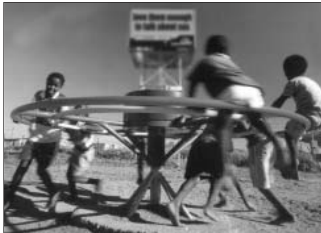
Roundabout play pump: combines the need for pumping with the fun of playing
