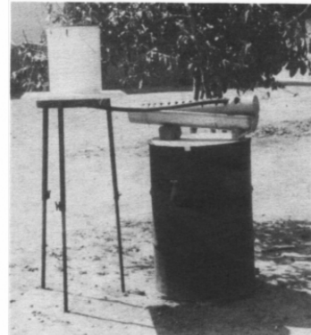
A completed iron removal unit in a homestead yard.
