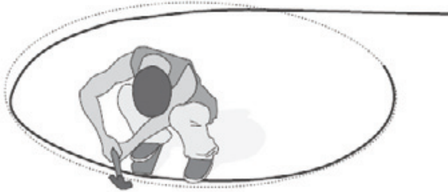
Fig. 15: Bending the horizontal hoops
