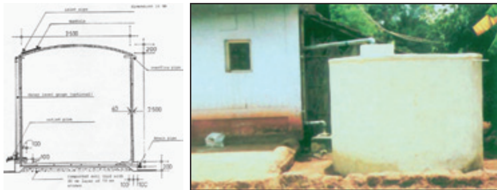
Figs. 4–5: Cylindrical ferrocement tanks
