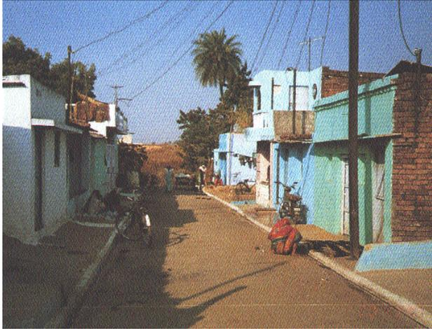
Roads Have positively downward slopes from high points to drainage courses and are thus able to act as storm water channels and attenuate the rain peaks.
