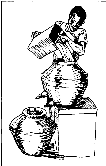
Pouring turbid water into the first pot for treatment
