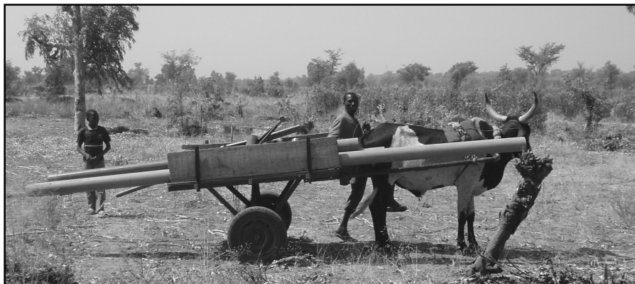
Hand auger equipment can be transported cheaply by ox cart
