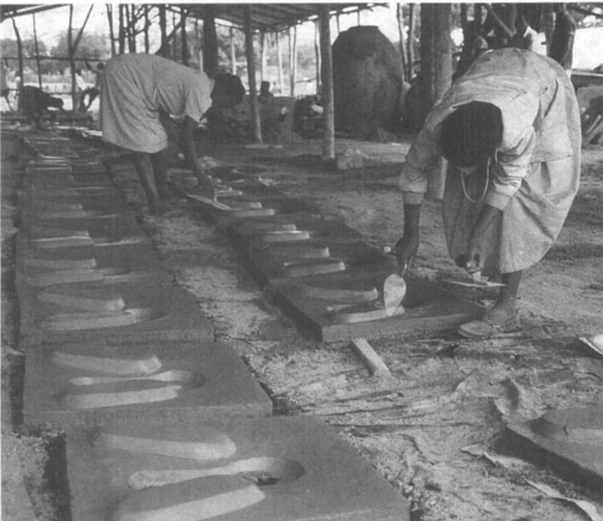
The RUWASA project in Uganda, where women from the African Housing Fund are producing over 1000 sanplats a month.
