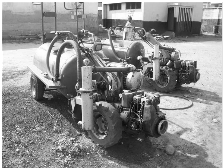
Dung Beetle machines owned by Larsen Ghana are small enough to enter the narrow lanes
