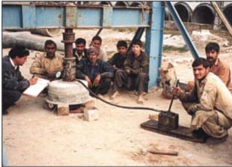
Figure 2-16 Bearing test rig for covers
