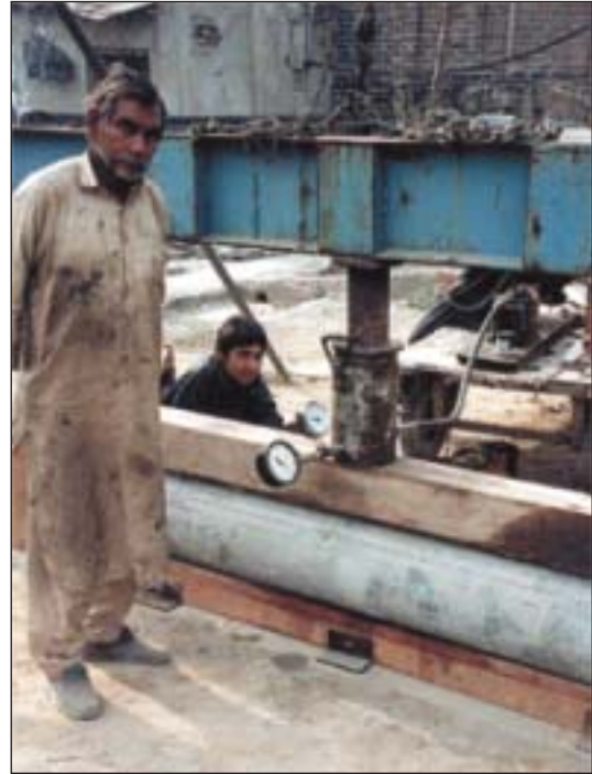
Figure 2-5 Three-edge bearing tests
