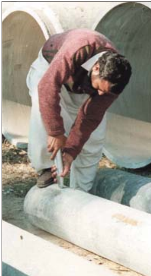
Figure 2-8 Schmidt hammer test
