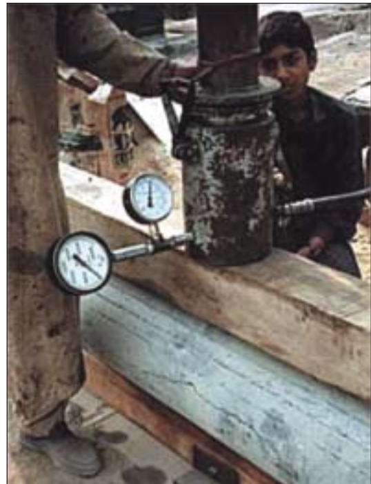
Figure 2-6 Loading of pipe to achieve 2mm wide crack (secondary gauge)
