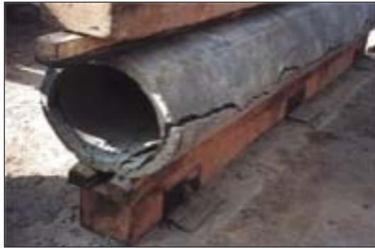
Figure 2 7 Substantial deformation of pipe without collapse
