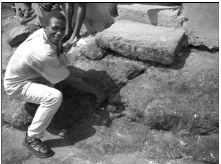
Geological reconnaissance includes spotting surface fissures
