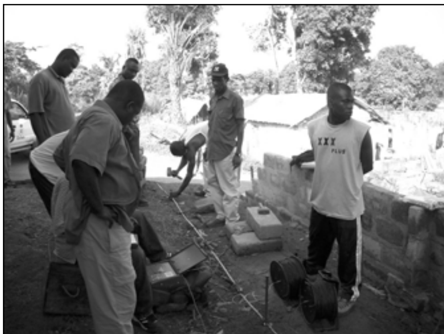
Taking resistivity readings
