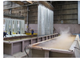
Counter-current rinsing can typically be used in electroplating operations.
