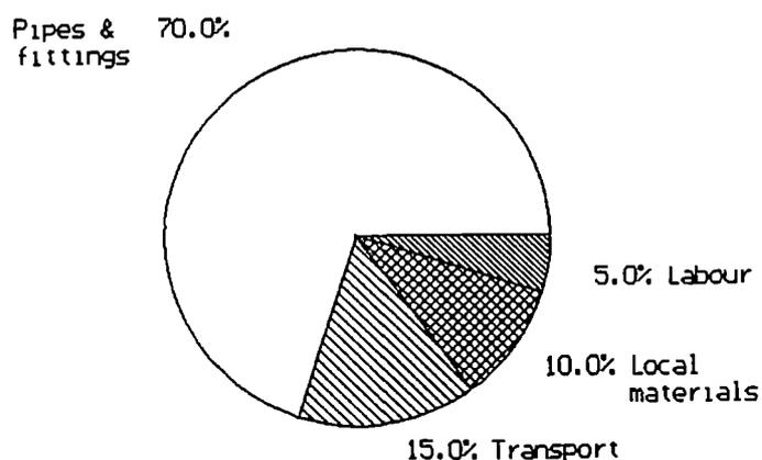
Figure 3. Capital cost distribution for gravity piped schemes.
