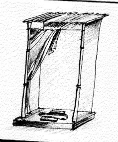
as bamboo matting, old drums, rubble masonry work, etc, can also be used for pit lining to reduce the cost. Place the squatting slab over the pit, once the pit is ready. Use a spirit level to check the horizontal level of the slab. If the horizontal level is not achieved, the required waterseal will not be ensured and the latrine will not function properly.
