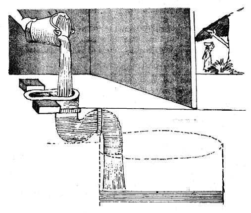
water. The water present in the bent pipe works as a water seal. Excreta is flushed by water through this water seal into the pit. For this, a bucketful of water is always necessary for flushing the excreta into the pit.
