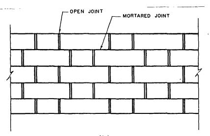
Note:ALL EXPOSED VERTICAL JOINTS OPEN WHILE THE REST LAID IN CEMENT SAND MORTAR
