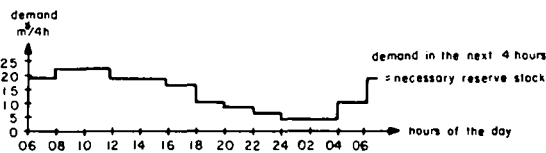
Fig. 10.2 Minimum reserve: 2nd diagram: Integral over 4 hours = necessary minimum storage
