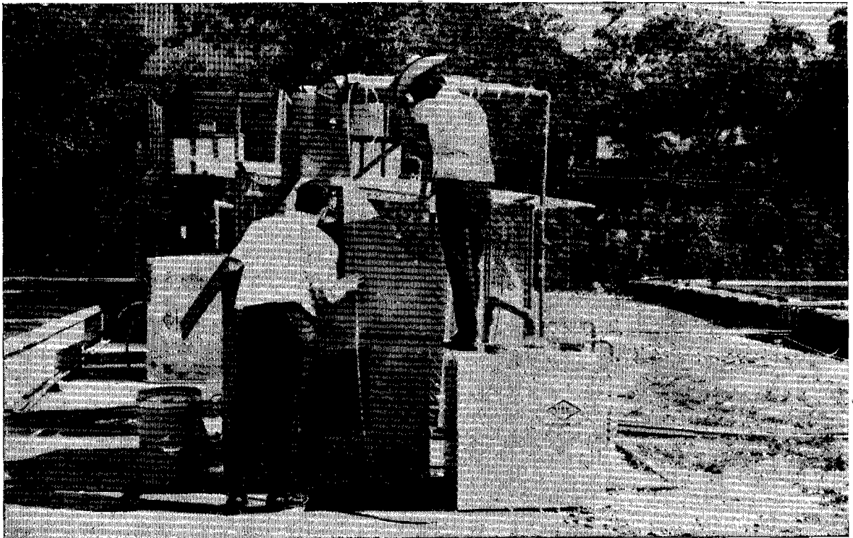
Fig. 3—The Downflow Solids Contact Flotation Chamber Used to Harvest the Algal Cells.
