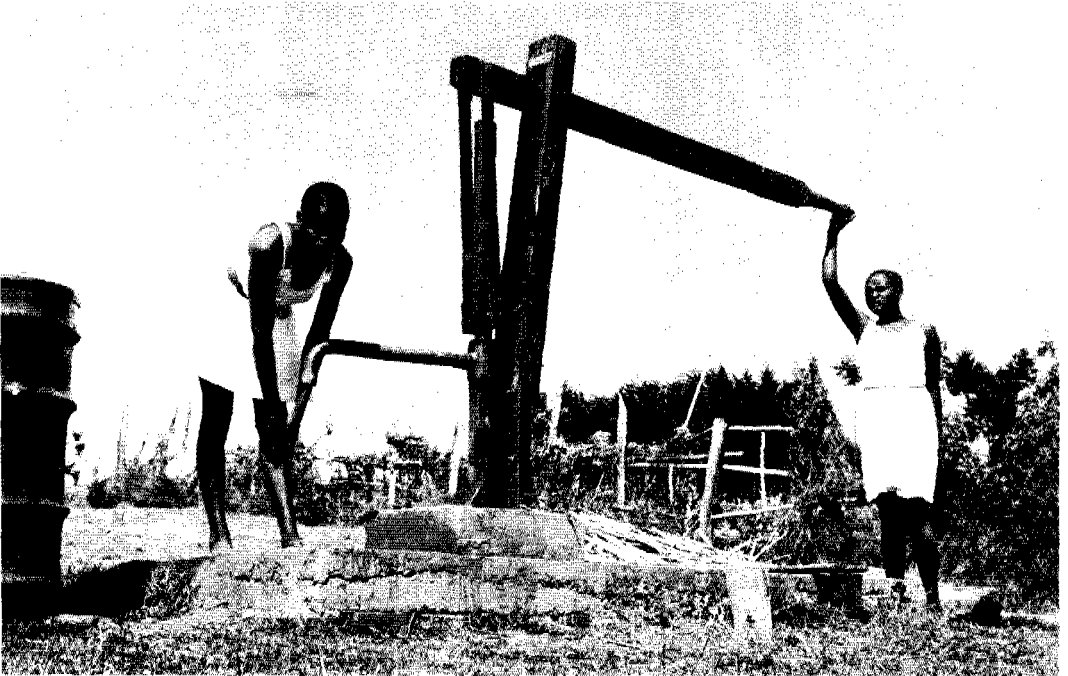
Locally Manufactured Hand Pump
