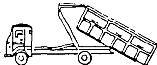
Container being pulled on to truck
