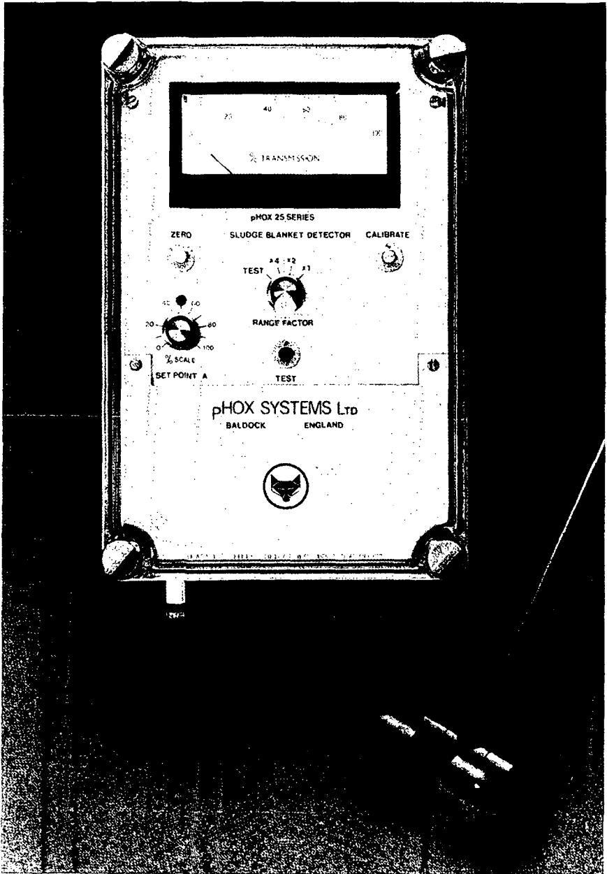
Plate 12. Example of an optical sludge level detector.
