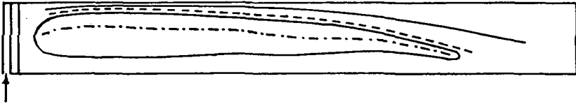
Fig. 27. Horizontal flow pattern in primary tank at Rotherham, determined by two-float technique
