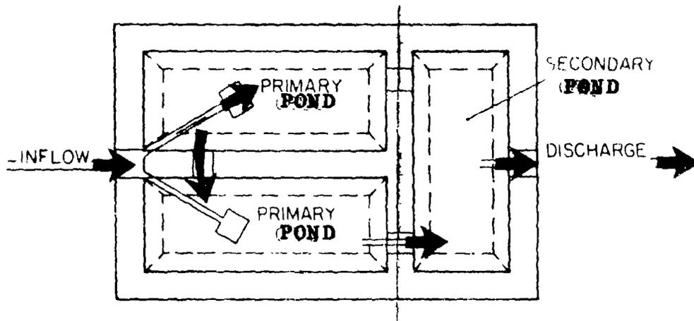
Fig. 8.2 Diagram shows ponds in series
