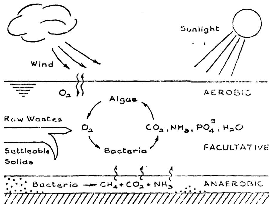
**Fig. 5.3** WASTE STABILIZATION POND MECHANISMS
