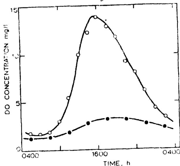
**Fig. 5.4** Diurnal variation in dissolved oxygen,  $\circ$ , top 200 mm of pond,  $\bullet$ , 800 mm below surface
