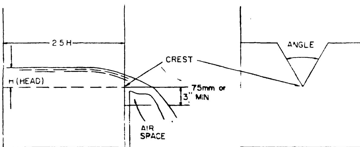
To determine flow, measure the head of water above the crest of the weir. Then use the chart on the following page to determine flow in metric units.
