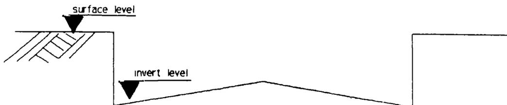
Figure 13: Cross section road. The surface level is the ground level next to the road. The invert level is the lowest point of a cross section of a road.
