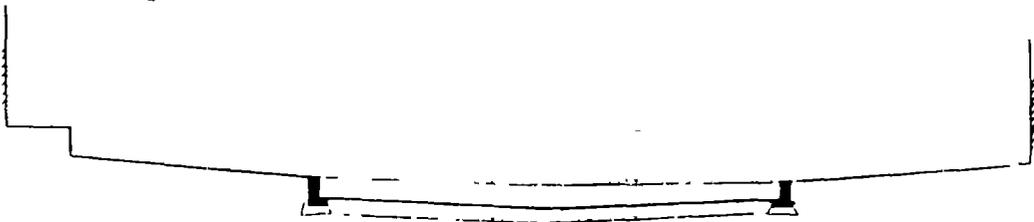
The RSD consists of paved roads with kerbstones so high, that the maximum water levels caused by the design rainfall, will be just below the top of the kerbstone.
