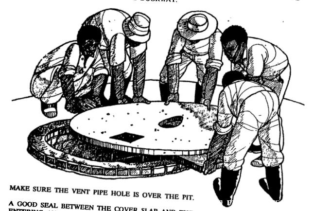
A GOOD SEAL BETWEEN THE COVER SLAB AND THE COLLAR PREVENTS FLIES FROM ENTERING AND LEAVING THE PIT OTHER THAN THROUGH THE SQUAT AND VENT PIPE HOLES.
