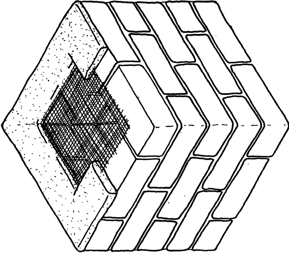
Figure 7. Attachment of flyscreen to brick vent pipe.
