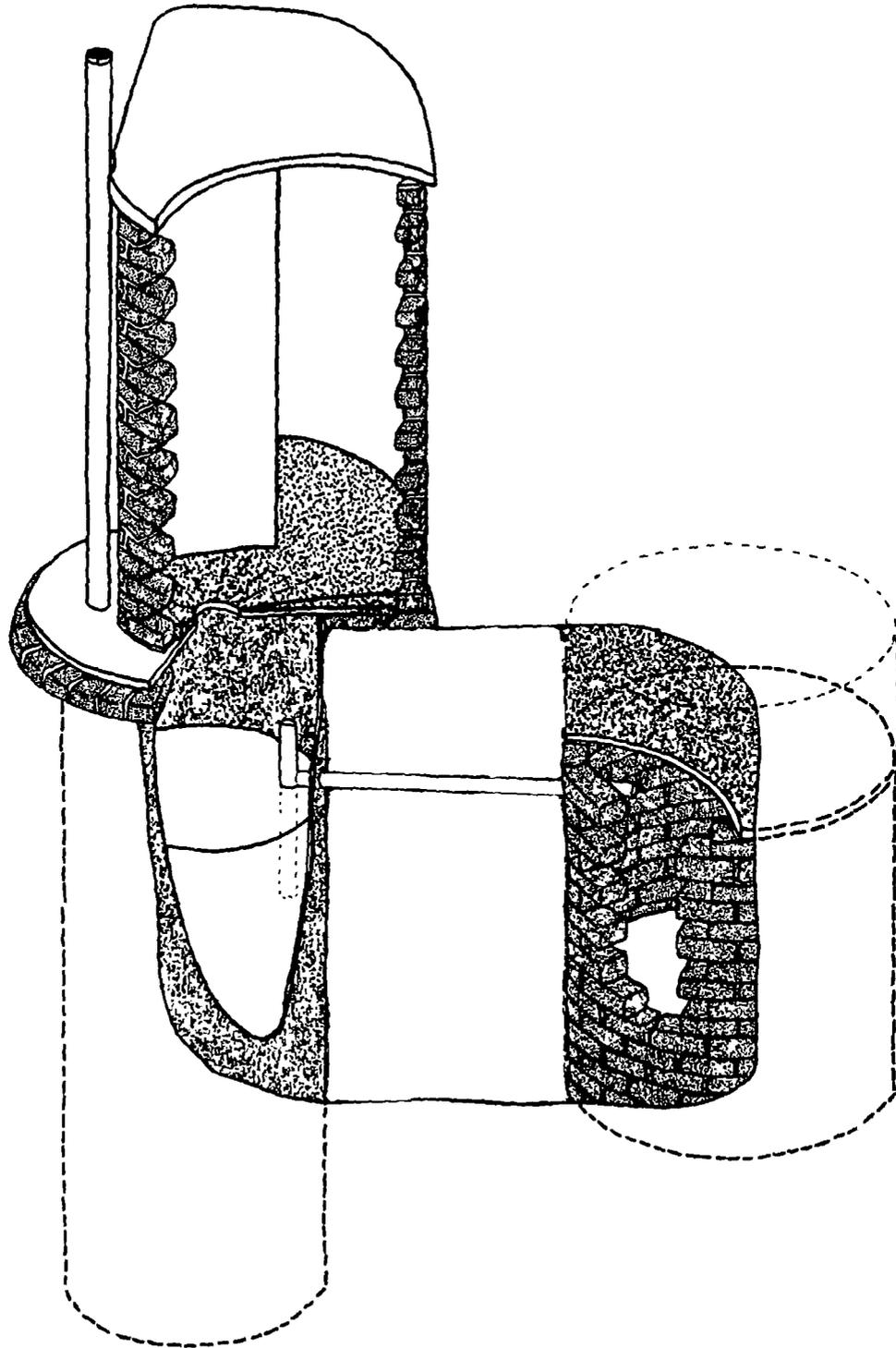
Figure 10. Schematic diagram of VIP latrine with soakaway.
