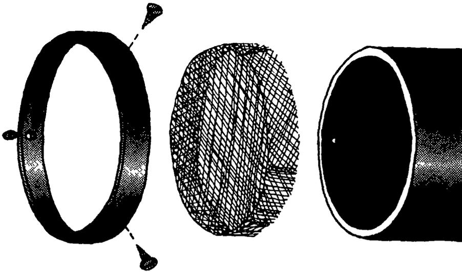
Figure 6. Attachment of flyscreen to PVC vent pipe.
