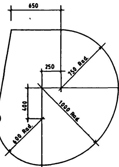
CONCRETE ROOF SLAB FOR ROUND SPIRAL SUBSTRUCTURE
