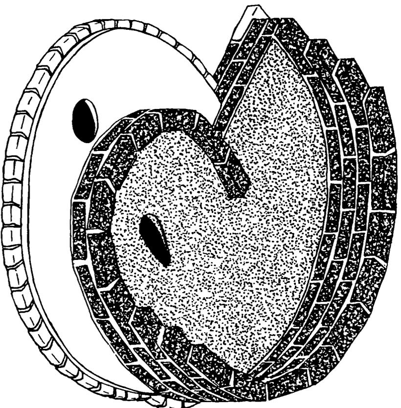
Figure 5. Isometric sketch of a brick VIP latrine during construction.
