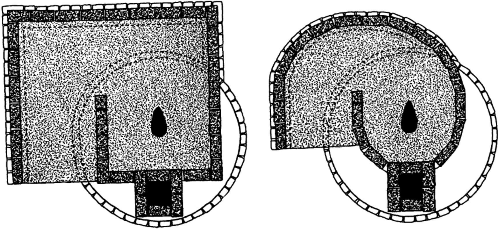
Figure 4. Alternative shapes of spiral superstructure for VIP latrines.
